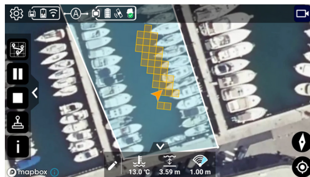
View of a bathymetric survey of Cassis harbor on the remote control of the Jellyfishbot
