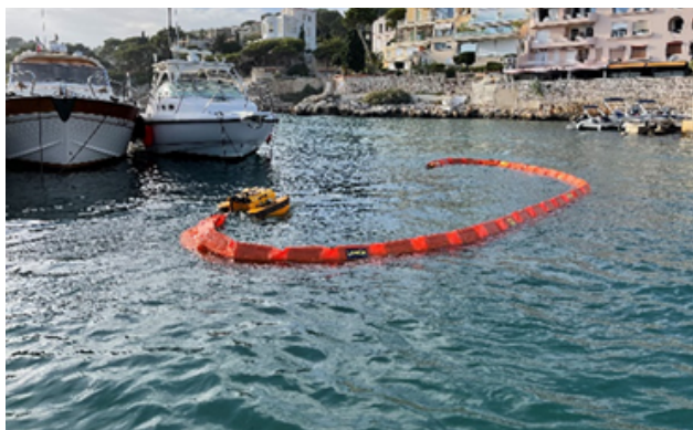
The Jellyfishbot deploying the Harbo boom
