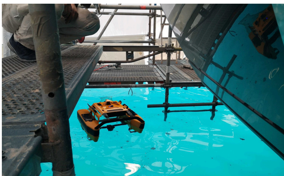
The Jellyfishbot collecting paint dust
